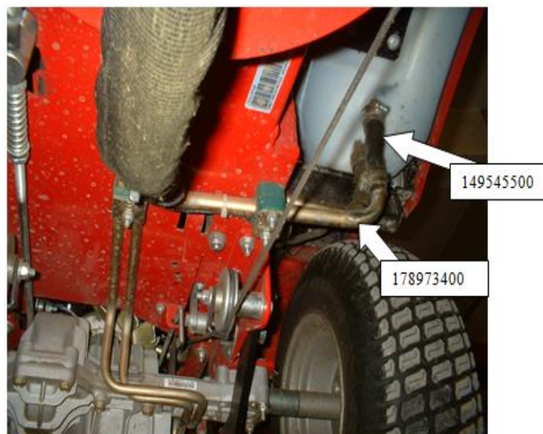
Figure 4: Oil Return pipes
