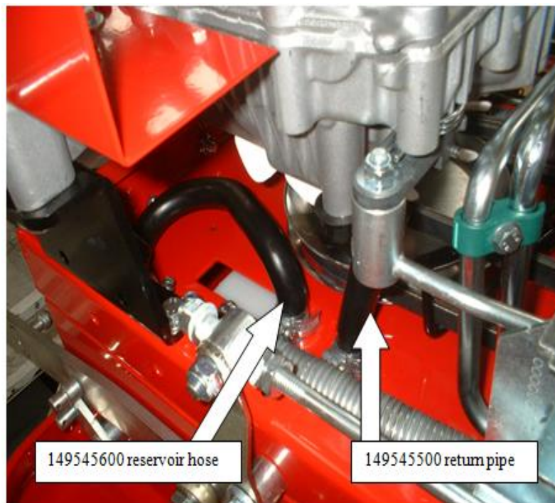
Figure 5: Oil Tank Flexible pipes
